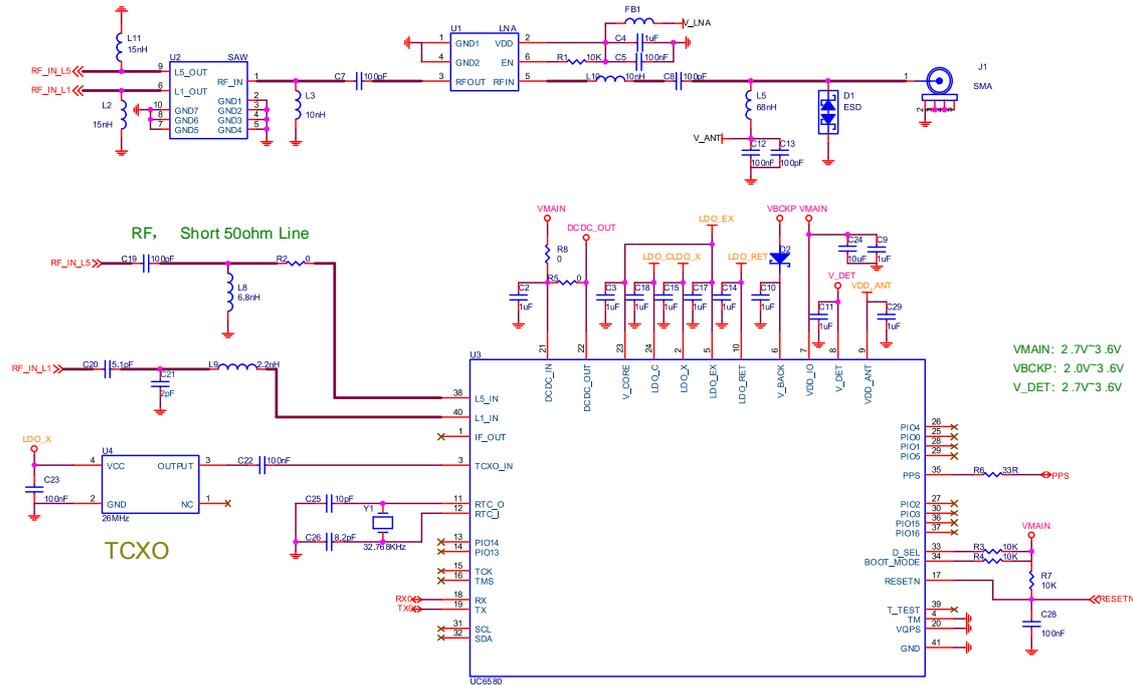
Figure 1-1 Reference design of LDO mode
